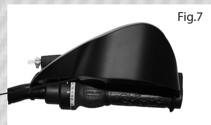
Tornado shield secured with brake angled down
