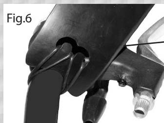
Tornado shield secured with brake horizontal
